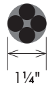
1¼" solid rope maximum length is 228 inches use ring with minimum 1¾"ID
