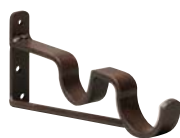
DBL1 custom steel double bracket please specify: A. front pole size and profile B. back pole size and profile C. rings to be used, if any D. front and back returns (distance from wall to center of cradle) note: returns are contingent upon which poles and rings are chosen 3½"H backplate comes standard, unless otherwise specified
