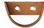
IM175 inside mount steel bracket for poles up to 1 3/8"-1 3/4" Dia 1 1/2" backplate, 3/4" deep, 2 1/4"W
