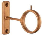
EB5 steel eyelet bracket, single 3 1/2" backplate, 3 1/2" return, eyelet 1 7/8" ID
