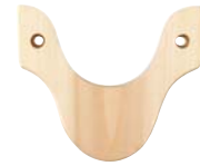
ISM inside wood mount bracket for poles 2", 2 1 / 4 " Dia 3 1 / 2 " backplate, 1" deep, 4 1 / 8 " W
